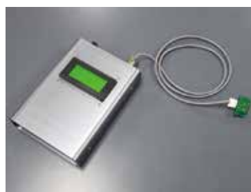
Figure 2. Magnetic field measurement instrument.
