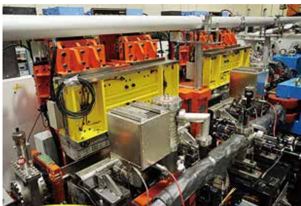
Figure 2. Twin Polarization-variable Undulators/Optical Klystron at UVSOR-III.
