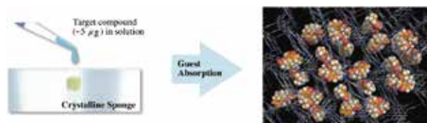
Figure 3. Schematic representation of crystalline sponge method.
