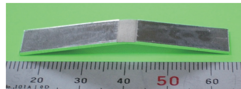
Figure 3. Example of bend workpiece (A1100, t = 1 mm).
