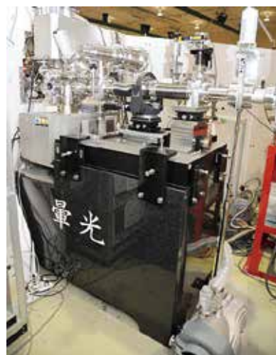
Figure 3. Optical Cavity for Resonator Free Electron Laser is under reconstruction at UVSOR-III.
