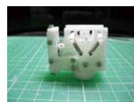
Figure 2. Prototype model of the equipment for crystal bending generated by 3D printer.
