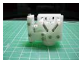
Figure 2. Prototype model of the equipment for crystal bending generated by 3D printer.
