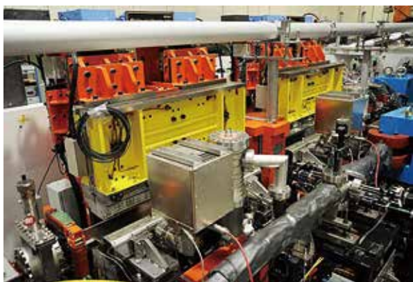
Figure 2. Twin Polarization-variable Undulators/Optical Klystron at UVSOR-III.
