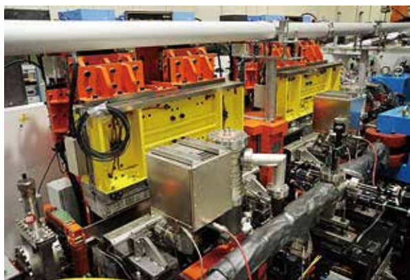
Figure 2. Twin Polarization-variable Undulators/Optical Klystron at UVSOR-III.
