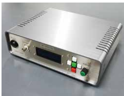
Figure 2. High voltage amplifier for driving bimorph pump.
