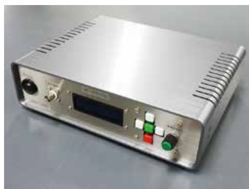
Figure 2. High voltage amplifier for driving bimorph pump.
