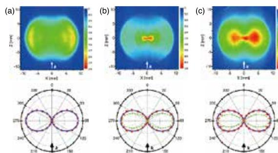
**Figure 2.** Photoelectron angular distributions of helium atoms measured for the (a) first, (b) second and (c) third harmonics from helical undulator. The solid blue curves represent fits assuming electric dipole transition. The dotted green curves in (b) and (c) show the angular dependence of the photoelectron expected for non-dipole transitions induced by the OAM carried by the VUV vortex.
