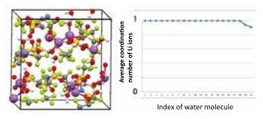
The mechanism of hydrate-melt electrolytes for high-energy-density aqueous batteries, was found computationally in this project. (Left) schematic picture of equilibrium state of newly-developed hydrate melt, (Right) coordination number of Li ions from each water molecule. *Nat. Energy* **1**, 16129 (2016).
