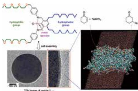
**Figure 3.** A self-assembled vesicular palladium NCN-pincer complex.
