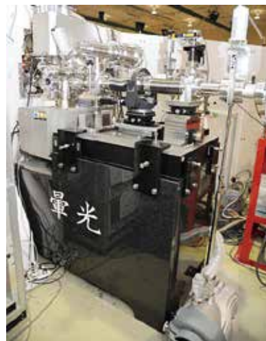
Figure 3. Optical Cavity for Resonator Free Electron Laser.
