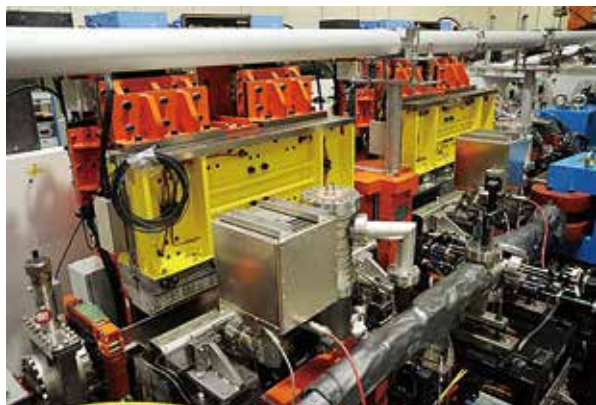
Figure 2. Twin Polarization-variable Undulators/Optical Klystron at UVSOR-III.
