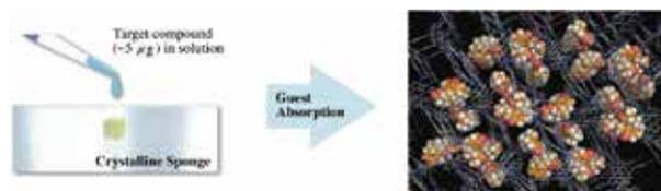
**Figure 3.** Schematic representation of crystalline sponge method.
