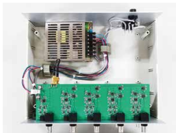
Figure 2. Inside view of Signal Fan-out Buffer and Distributor.
