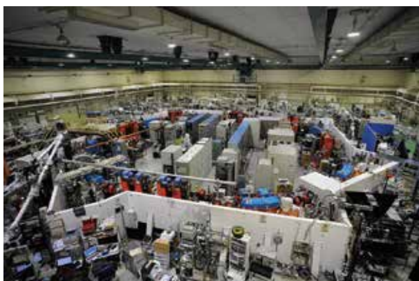
Figure 1. UVSOR-III electron storage ring, radiation shield wall, and beamlines/endstations.
