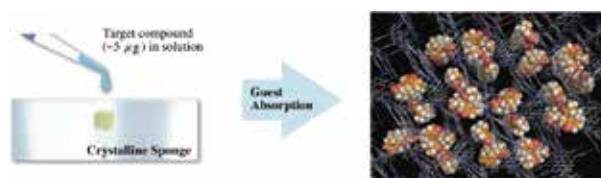
Figure 3. Schematic representation of crystalline sponge method.
