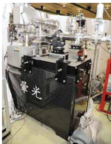
Figure 3. Optical Cavity for Resonator Free Electron Laser.
