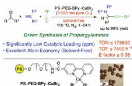
Figure 4. Preparation of Propargylamines by A 3 Coupling Reaction with ppm Loading Level of a Polymeric Cu(II) Catalyst.
