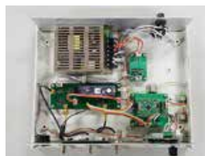
Figure 2. Inside of a Delayed Pulse Generator (1ch version).
