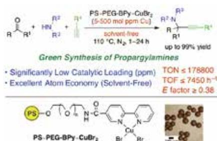
**Figure 4.** Preparation of Propargylamines by A<sup>3</sup> Coupling Reaction with ppm Loading Level of a Polymeric Cu(II) Catalyst.
