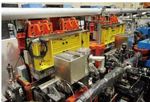
**Figure 2.** Twin Polarization-variable Undulators/Optical Klystron at UVSOR-III.
