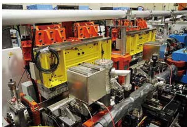
Figure 2. Twin Polarization-variable Undulators/Optical Klystron at UVSOR-III.
