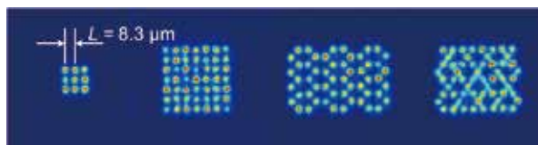
Figure 4. Examples of arbitrary optical trap arrays generated with a low NA convex lens ( L = 8.3 \mu\text{m} ; wavelength = 633 nm; NA = 0.0446), corresponding to L = 640 nm with NA = 0.75 at the wavelength 820 nm. 3)
