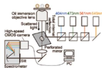
**Figure 3.** Spectrometer-based multi-color dark-field imaging system.
