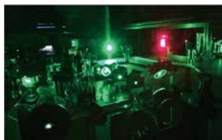
Figure 1. Setup for advanced ultrafast spectroscopy based on sub-10-fs pulses.
