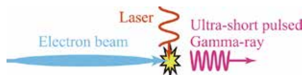
Figure 1. Schematic illustration of 90-degree laser Thomson scattering.
