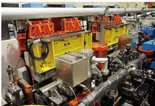
Figure 2. Twin Polarization-variable Undulators/Optical Klystron at UVSOR-III.
