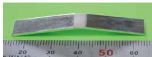
Figure 3. Example of bend workpiece (A1100, t = 1 mm).
