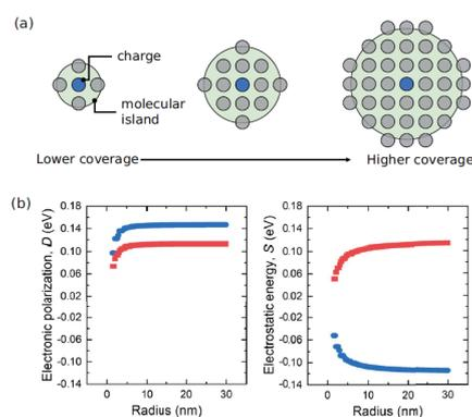
**Figure 3.** (a) Disk model for the growing island without a changing lattice constant. (b) Calculated polarization energy and electrostatic energy for ZnPc and  $F_{16}$ ZnPc are indicated with blue circles and red squares. The figure is after ref 2).
