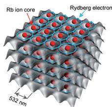
**Figure 2.** Schematic of the standard hardware of the ultrafast quantum simulator.<sup>3,4,6,7,10)</sup>
