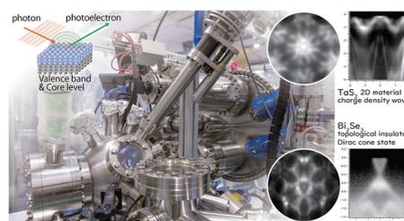
**Figure 1.** Photoelectron momentum microscope at BL6U of UVSOR synchrotron facility together with valence photoelectron holograms and dispersions of  $\text{TaS}_2$  and  $\text{Bi}_2\text{Se}_3$ . Charge density wave phase transition and topological nature can be directly studied in detail.
