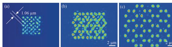
**Figure 3.** Examples of the world’s smallest arbitrary arrays of optical traps. (a) Square lattice; (b) Kagome Lattice; (c) Hexagonal (Honeycomb) lattice.<sup>10)</sup>
