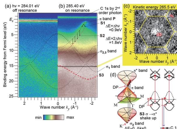
**Figure 3.** Momentum-resolved valence photoelectron and Auger electron spectra along the direction excited at the photon energy of (a) 284.01 eV and (b) 285.40 eV. Black and red dotted lines indicate the valence band and Auger electron dispersions, respectively. (c) Iso-energy momentum-resolved Auger electron intensity distribution at the kinetic energy of 266.5 eV. (d) Schematic of resonant Auger-electron emission for the pathway S3.<sup>3)</sup>
