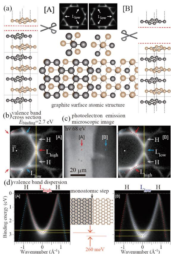
**Figure 2.** (a) Atomic structure of the cleaved graphite surface. (b) Iso-energy cross section of the graphite surface  $\pi$  band. (c) Graphite single atomic layer step was imaged with different contrast owing to the difference in the  $\pi$  band binding energies in two different terraces as shown in (d).<sup>2)</sup>
