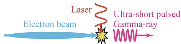
**Figure 1.** Schematic illustration of 90-degree inverse Thomson scattering.
