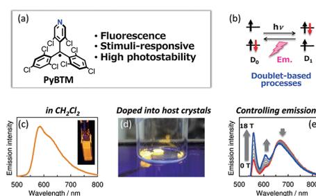
**Figure 1.** (a) Molecular structure of PyBTM and its characteristics. (b) Schematic photoexcitation-emission processes. (c) Emission in CH<sub>2</sub>Cl<sub>2</sub>. (d) Emission of PyBTM-doped molecular crystals. (e) Controlling emission by magnetic field.
