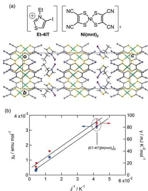
**Figure 2.** (a) Chemical and crystal structures of (Et-4IT)[Ni(mnt)<sub>2</sub>]<sub>2</sub>. (b)  $\gamma$ - $J^{-1}$  and  $\chi_0$ - $J^{-1}$  plots for organic QSLs.
