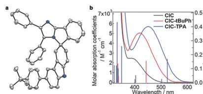
**Figure 4.** (a) ORTEP representation of **CIC-tBuPh** with thermal ellipsoids (50% probability), where the nitrogen atom is highlighted in blue. Hydrogen atoms and solvent molecules are omitted for clarity. (b) Steady-state absorption spectra of **CIC**, **CIC-tBuPh** and **CIC-TPA** in benzene at room temperature. Vertical lines indicate the theoretical spectra of each molecule.
