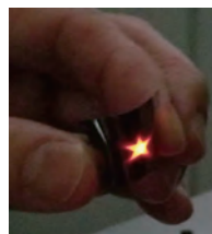
Figure 1. Up-converted (UC) yellow emission by star-shaped near infrared irradiation.
