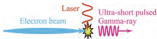
Figure 1. Schematic illustration of 90-degree inverse Thomson scattering.
