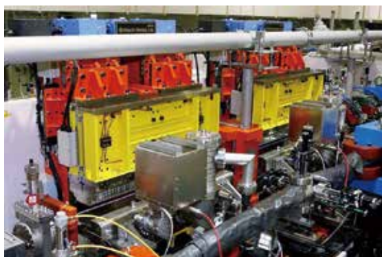
Figure 2. Twin Polarization-variable Undulators/Optical Klystron at UVSOR-III.
