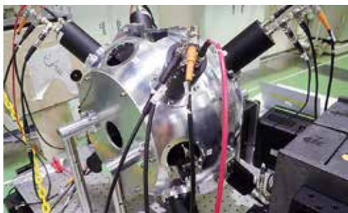
Figure 2. Positron annihilation lifetime measurement system using eight detectors and two digital oscilloscope.
