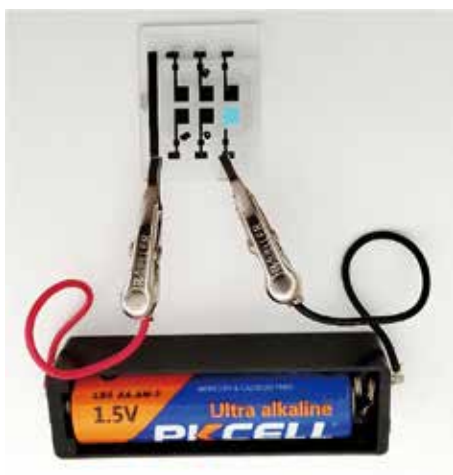
Figure 4. Lighting up a blue organic LED with a single 1.5 V battery.
