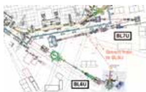
Figure 1. Schematic view of beamlines BL7U and BL6U. The low-energy photon of BL7U will be introduced to BL6U for multimodal experiments.
