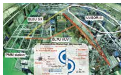
Figure 1. Photoelectron momentum microscope station at UVSOR synchrotron facility. Soft X-rays from BL6U for k_z dispersion and core-level excitations and vacuum ultraviolet light from BL7U at normal incidence for atomic orbital analysis make this station unique.
