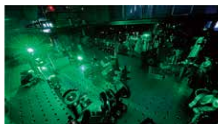
Figure 1. Setup for advanced ultrafast spectroscopy based on sub-10-fs pulses.
