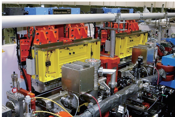
Figure 2. Twin Polarization-variable Undulators/Optical Klystron at UVSOR-III.
