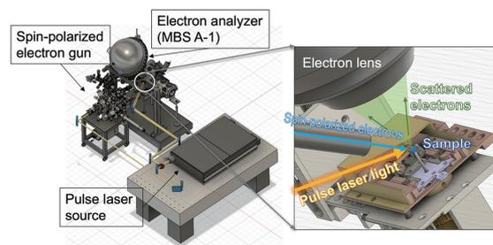
**Figure 1.** Time-, Spin-, and Angle-Resolved resonant Electron-Energy-Loss Spectroscopy (tSAR-rEELS) apparatus, which our group is now developing. The apparatus comprises a high-brilliant spin-polarized electron gun, a photoelectron spectrometer, and a femto-second pulse laser with an optical parametric amplifier.
