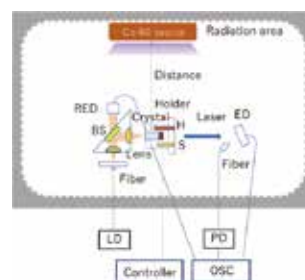
Figure 4. Experimental setup (BS: beam splitter; controller: temperature controller; crystal: YAG crystal; ED, RED: energy detector; fiber: optical fiber; H: heater; holder: specimen holder; LD: laser diode; lens: lens; OSC: oscilloscope; PD: photodiode; S: temperature sensor).
