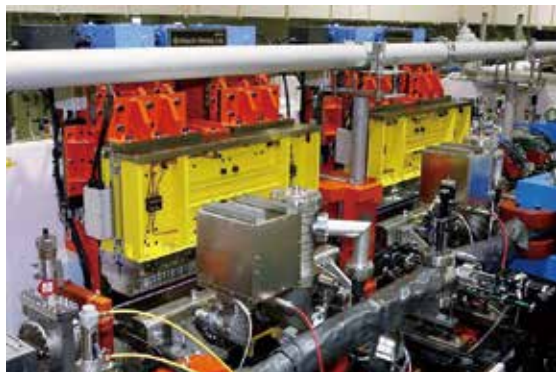
Figure 2. Twin Polarization-variable Undulators/Optical Klystron at UVSOR-III.
