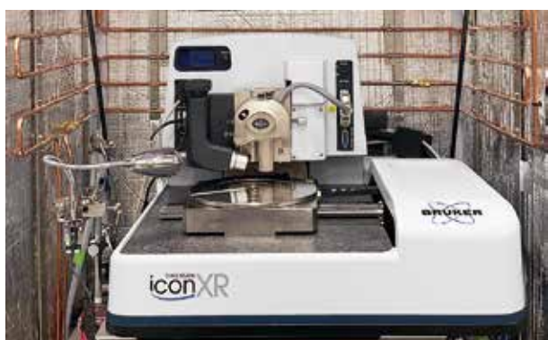
Figure 2. The Bruker microscope at the Instrument Center devised for operation at −10 °C.
