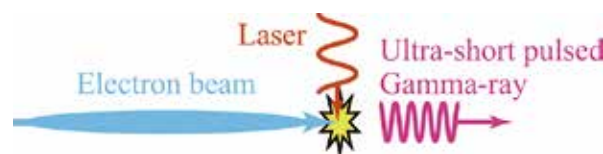
Figure 1. Schematic illustration of 90-degree inverse Thomson scattering.
