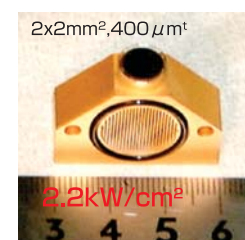
Microchip laser developed at the center.
