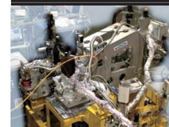
Next generation soft X-ray emission spectrometer developed at UVSOR.
