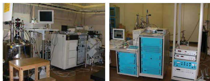
(Left) Multi-frequency pulsed-ESR Spectrometer, Bruker E680. (Right) Pulsed FT-NMR Spectrometer.
