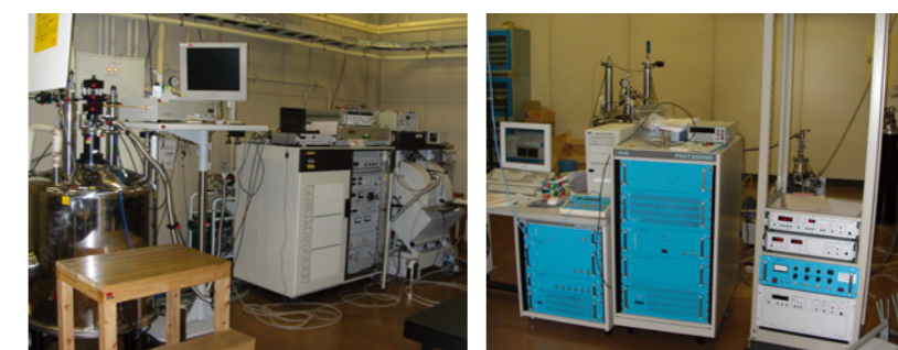
(Left) Multi-frequency pulsed-ESR Spectrometer. (Right) Pulsed FT-NMR Spectrometer.
