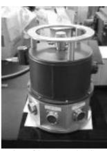
Figure 1. Outer view of 256-channel MCT photoconductive array cell.
