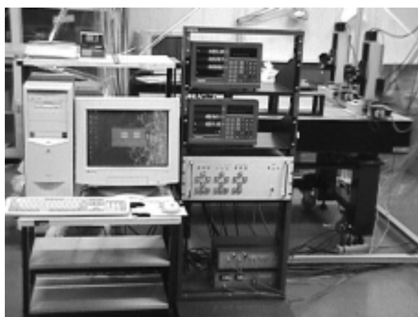
Figure 3. Driver for linear translation stage and host computer.
