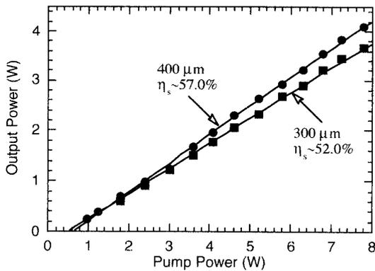
Figure 1. Output power as a function of pump-power.
