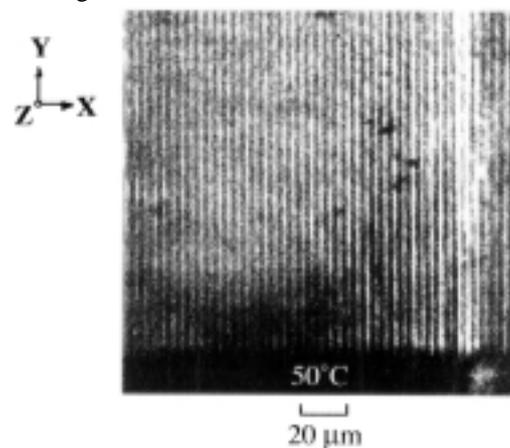
Figure 1. Photo of a Z-cut QPMLT device.
