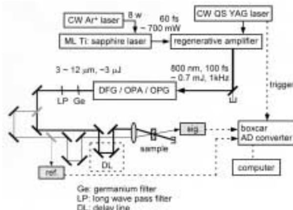
**Figure 1.** Apparatus for the femtosecond IR-IR pump-probe measurements.
