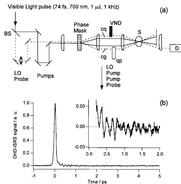
**Figure 1.** (a) Constructed apparatus of an OHD-ISRS measurement. (b) Optical heterodyne detected impulsive stimulated Raman scattering signal of liquid carbon tetrachloride measured using a phase mask. Inset: The signal in the early time region is depicted in a magnified scale.
