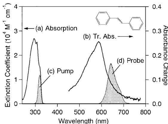
**Figure 1.** Spectral properties of *trans*-stilbene in the  $S_0$  and  $S_1$  states. (a) Steady-state absorption spectrum of *trans*-stilbene in heptane. (b)  $S_n \leftarrow S_1$  transient absorption spectrum of *trans*-stilbene in heptane measured at 1 ps after 267-nm photoexcitation. Spectra of the pump (c) and the probe (d) pulses used in the 40-fs-resolved absorption measurements are also shown.
