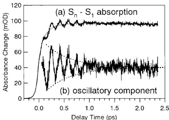
**Figure 2.** Time-resolved absorption signal of *trans*-stilbene in heptane ( $10^{-2}$  M). (a) Temporal behavior of the  $S_n \leftarrow S_1$  absorption (640 nm) measured with excitation at the reddest edge of the ground-state absorption (320 nm). (b) Oscillatory component depicted in a magnified scale.
