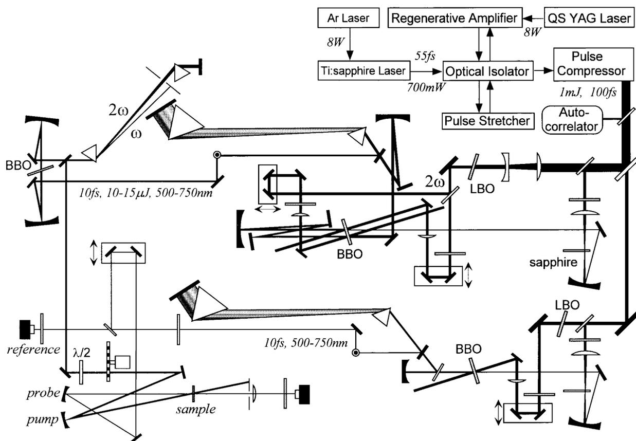
**Figure 1.** Experimental apparatus of the extremely-fast time-resolved absorption spectrometer using independently-tunable pump and probe pulses.
