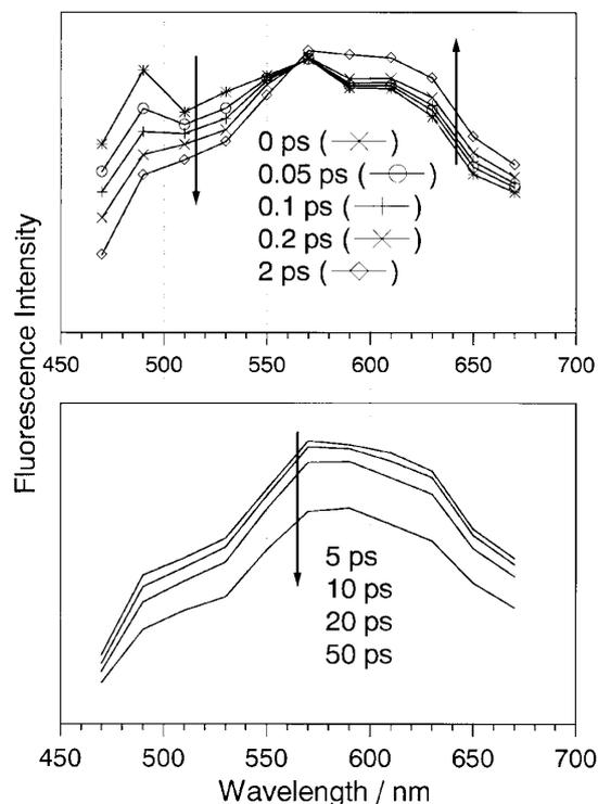
**Figure 1.** Reconstructed time-resolved fluorescence spectra of chrysazin. The spectra in the early time region are presented in the top panel. The spectra after 5 ps are presented in the bottom panel.
