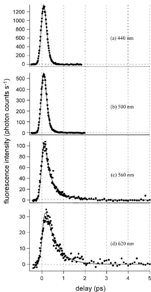
**Figure 1.** Time-resolved fluorescence of trans-azobenzene in hexane solution ( $5.0 \times 10^{-3}$  mol dm $^{-3}$ ) at 440 nm (a), 500 nm (b), 560 nm (c), and 620 nm (d). The dots are experimental data and the solid curves are the results of fitting analysis.
