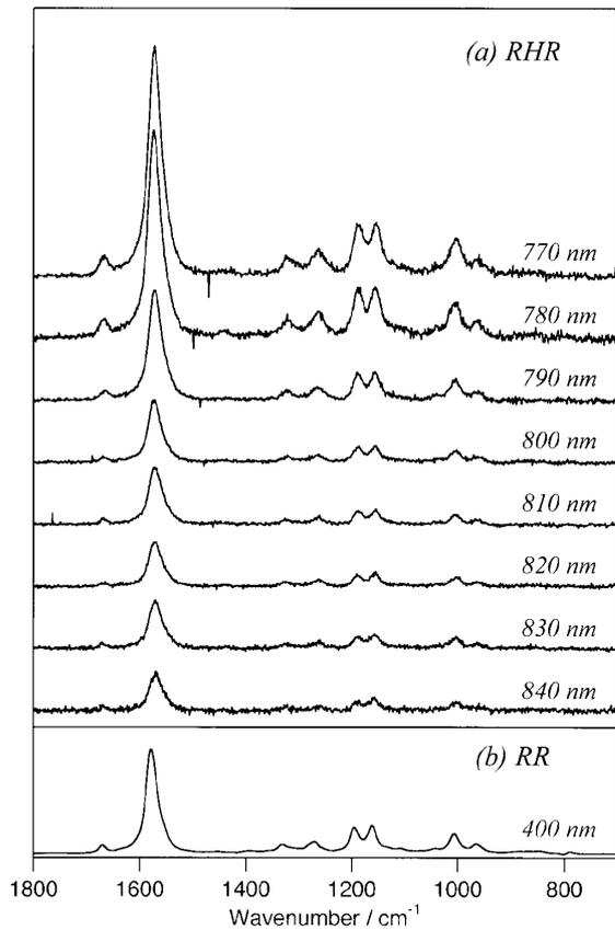
**Figure 1.** (a) Resonance hyper-Raman (RHR) and (b) resonance Raman (RR) spectra of *all-trans* retinal in cyclohexane ( $1 \times 10^{-3}$  mol dm $^{-3}$ ).
