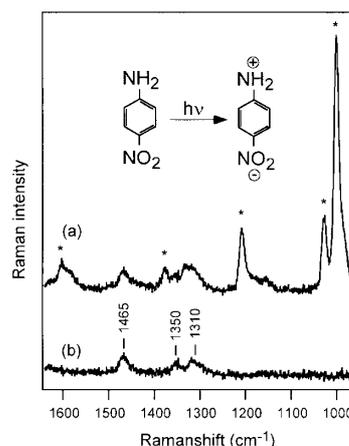
**Figure 1.** Picosecond time-resolved Raman spectra of *p*-nitroaniline in toluene solution ( $1.5 \times 10^{-2} \text{ mol dm}^{-3}$ ) at the delay time of 50 ps. Transient spectra (b) was obtained after the subtraction of the solvent (\*) and the ground state signals from (a).
