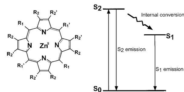
**Figure 1.** Molecular structure and schematic diagram of the relaxation processes of zinc(II) porphyrin.
