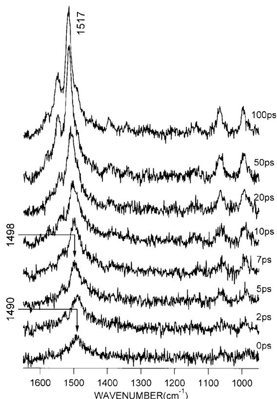
Figure 1. Picosecond time-resolved resonance Raman spectra of 5-dibenzosuberone in acetonitrile.
