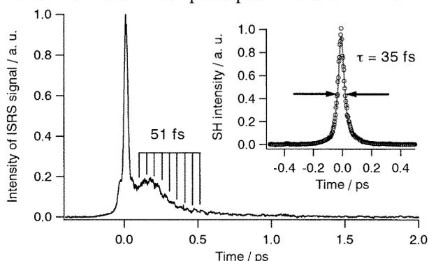
**Figure 1.** Impulsive stimulated Raman scattering signal of liquid  $\text{CS}_2$ . Inset: The autocorrelation of ultra short pulses that are used in this measurement.
