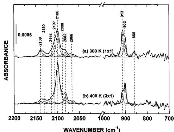
Figure 1. p-Polarized BML-IRRAS spectra associated with H/Si(100) surfaces with (a) 1×1 (b) 3×1. Narrow lines show peak-resolved spectra calculated assuming that the shape of each peak is Lorentzian.
