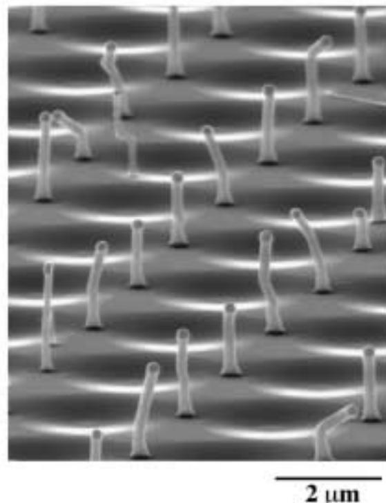
**Figure 1.** SEM image of Si pillars grown on Au-island arranged Si(111) substrates. The substrate was exposed to disilane gas of  $1 \times 10^{-2}$  Torr for 5 min at 620 °C. The angle of the electron beam incidence was 75°.
