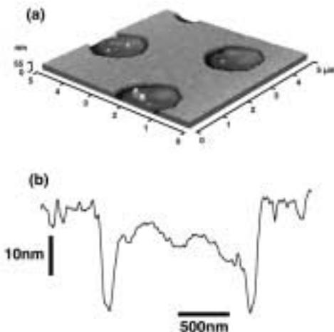
**Figure 1.** AFM observation of SiO<sub>2</sub> mask prepared by SR-stimulated etching. In (a) it is shown as a bird view image, and in (b) line profile near circular opening. Steep side wall is observed. However, surface is not smooth, against our expectation.
