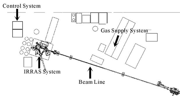
**Figure 1.** Schematic drawing of the BL4A2 beam line with the IRRAS system.
