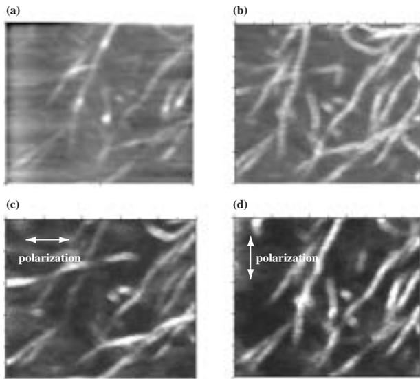
**Figure 1.** Observed images of J-aggregates (scan range  $5\ \mu\text{m} \times 5\ \mu\text{m}$ ). (a) Shear-force topography. (b) Unpolarized fluorescence image. (c) Horizontally and (d) vertically polarized fluorescence images.
