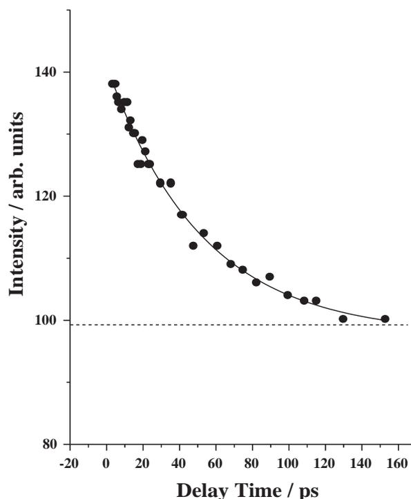
**Figure 1.** Near-field time-correlated PL signal of GaAs crystal.
