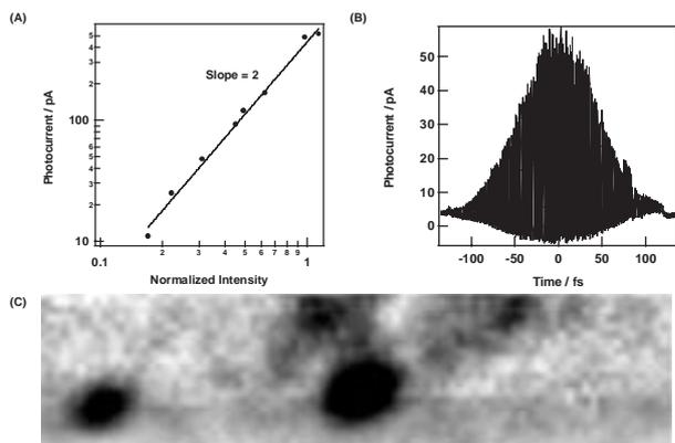
**Figure 1.** (A) Peak diode current as a function of normalized incident pulse energy. Solid line shows a quadratic fit to the data. (B) Autocorrelation signal obtained at the tip of the 100-nm apertured probe. (C) Spatial image (area size: 5  $\mu\text{m} \times 1.25 \mu\text{m}$ ) of photocurrent.
