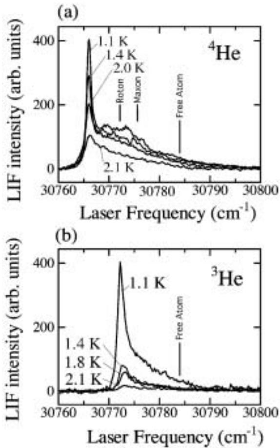
**Figure 1.** Excitation spectra of the  $4f^6(^7F)5d6s^2\ ^8F_{7/2} \leftarrow 4f^76s^2\ ^8S_{7/2}$  transition of Eu atoms in (a) liquid  $^4\text{He}$  and (b) liquid  $^3\text{He}$  at several temperatures.
