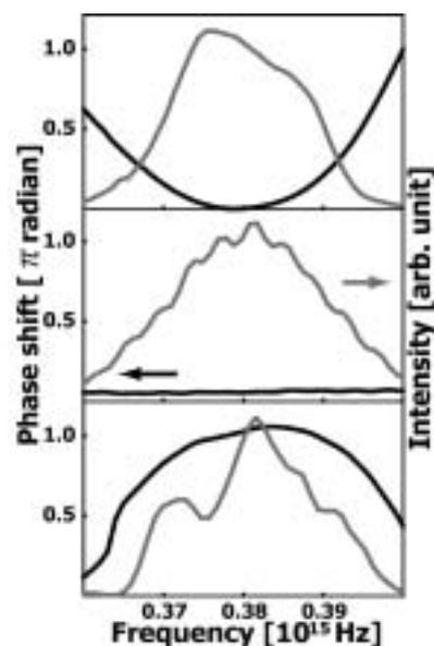
Figure 2. Spectra and phase dispersions of positively-chirped (top), transform-limited (middle) and negatively-chirped pulses (bottom).
