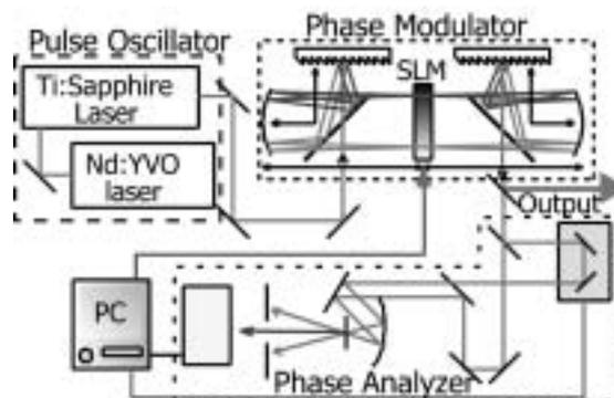
Figure 1. Schematic diagram of the phase-programmable femtosecond optical source.
