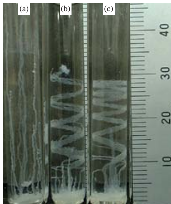
Figure 1. Magnetic field effects on the growth of zinc silicate membrane. (a) 0 T, (b) 6 T, (c) 13.5 T.
