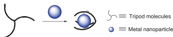
Figure 2. A schematic representation of the complex between the tripod molecule and the metal nanoparticle.
