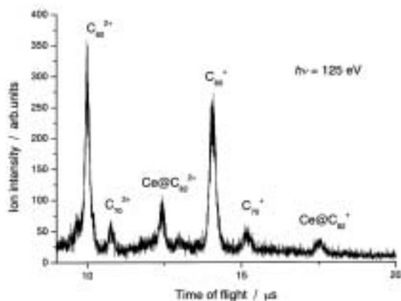
**Figure 1.** Time-of-flight mass spectrum of the parent and fragment ions produced by photoionization of Ce@C<sub>82</sub> at  $h\nu = 125$  eV.
