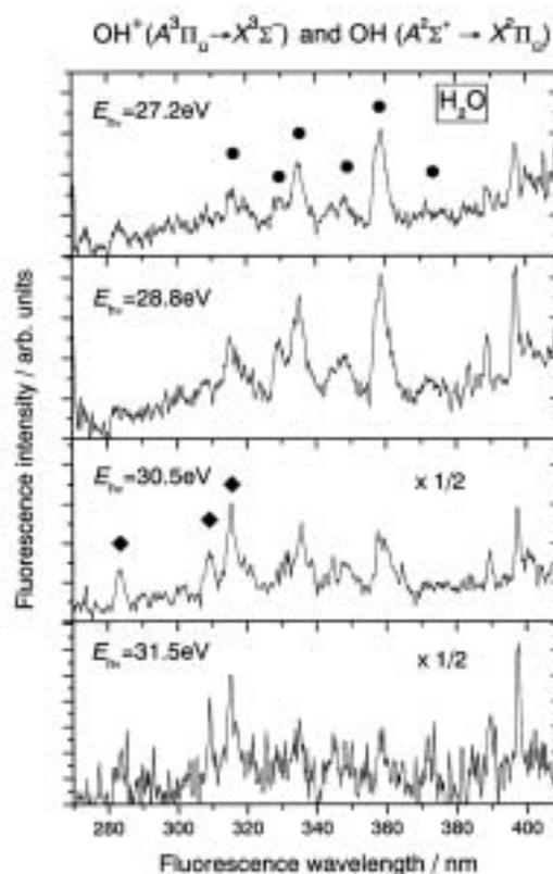
**Figure 1.** Dispersed fluorescence spectra of  $\text{H}_2\text{O}$ . The symbols  $\bullet$  and  $\blacklozenge$  designate the vibrational bands due to the  $\text{OH}^+(A^3\Pi \rightarrow X^3\Sigma^-)$  and  $\text{OH}(A^2\Sigma^+ \rightarrow X^2\Pi)$  transitions, respectively.
