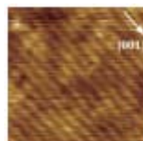
Figure 1. NC-AFM image of the TiO 2 surface (10 nm × 10 nm). The frequency shift and sample bias voltage were set at -186 Hz and 2 V, respectively.
