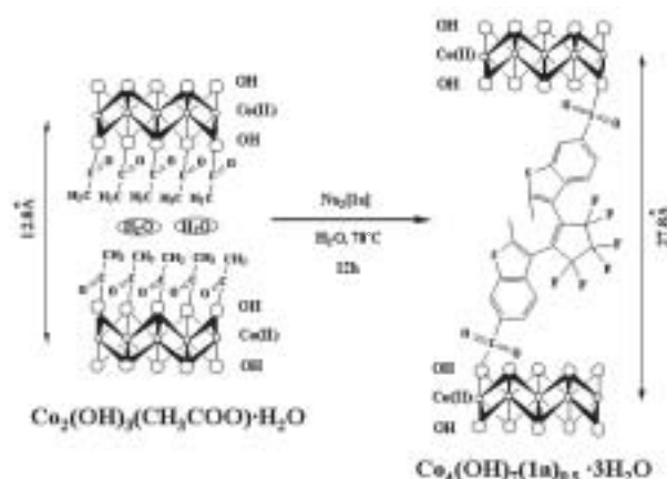
Figure 1. Schematic representation of the anion exchange reaction and the structure of 3 .
