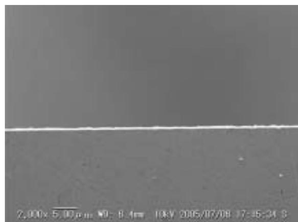
Figure 4. Top view of the slit blade observed by SEM.
