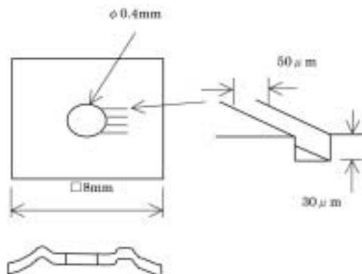
Figure 1. Schematic view of the metal gasket.
