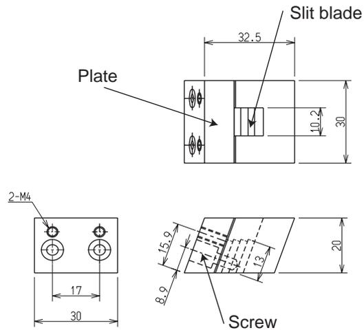
Figure 2. The clamp for the polishing of the edge surfaces.
