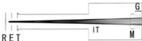
**Figure 1.** Schematic view of the momentum imaging spectrometer and simulated trajectories of  $C_{58}^+$  at initial kinetic energies of 0.1 eV. R, repeller; E, extractor; T, entrance electrode of a time-of-flight drift tube (TOF); IT, Ion trajectories; M, mass gate; G, ion reflector. The dimensions of all the electrodes are determined from the SIMION 3D software.
